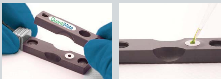
QuantiMate 200 cuvette, 0.2 mm path length, \pm 5\mu\text{m} accuracy, Z height = 15 mm, PN# 80-7100-71. Second image shows a sample being added to the cuvette for measurement
