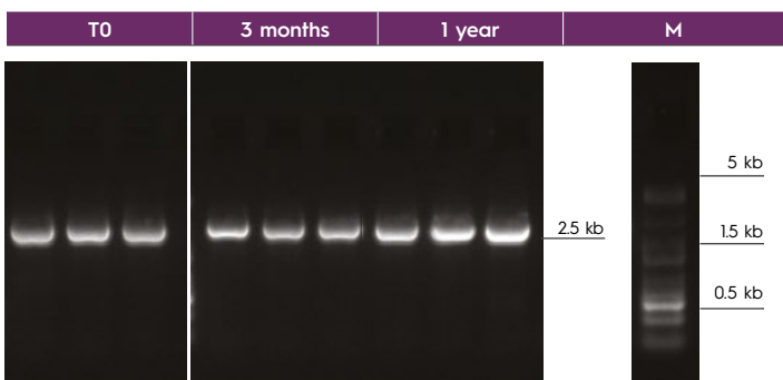
Agarose gel analysis (1XTAE, 1% agarose) of a direct amplification of a 2.5 kb PCR product from 1 mm discs taken from the center of dried saliva spot collected on GenCollect™ Color 2.0 card and stored 3 months or 1 year* at ambient temperature.
